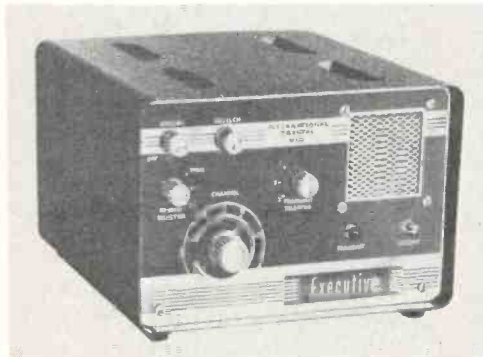
Tried and true, The International Crystal EXECUTIVE 100 shown with the EXECUTIVE model 23-channel frequency synthesizer. The EXEC 100 contains a number of deluxe features, with the dual conversion plus-crystal-filter receiver being especially good. A speech clipper accessory is also available.
